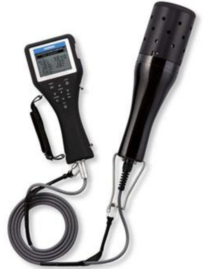
Limnological variables with water probe (DO, ORP, TDS, pH, K, Temperature, Turbidity)
