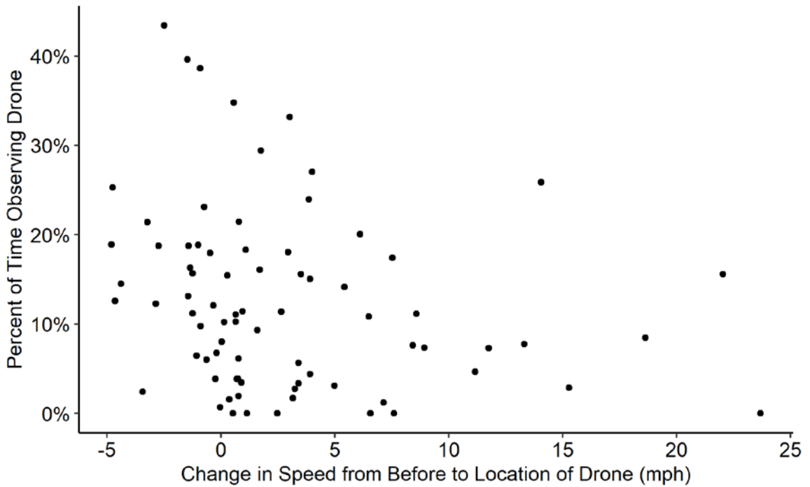
Figure 15: Relationship between the percent of time observing drone in the drone only scenarios and change in speed
