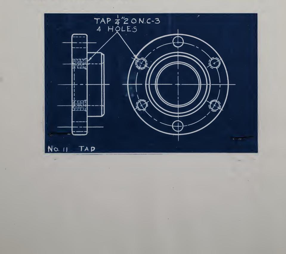
PART NO. 2001 PART NAME Adapter DEPT NO. H.S.T.S. MATERIAL Grinding O.D.OPER.NO.12 SHEET NO.1 NO.SHEETS 24 TYPE OF MACHINE Cylindrical grinder
