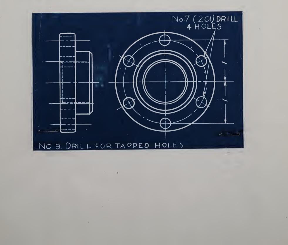
PART NO.2001 PART NAME Adapter DEPT NO. H.S.T.S. Recessing and MATERIAL burring OPER.NO.10 SHEET NO. 1 NO.SHEETS 24 TYPE OF MACHINE Drill press
