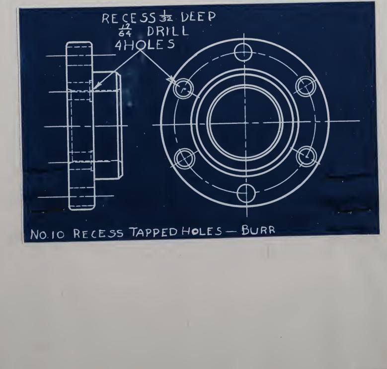
PART NO. 2001 PART NAME Adapter DEFT. NO. H.S.T.S. MATERIAL Hand tapping OPER.NO.11 SHEET NO.1 NO.SHEETS 24 TYPE OF MACHINE Bench
