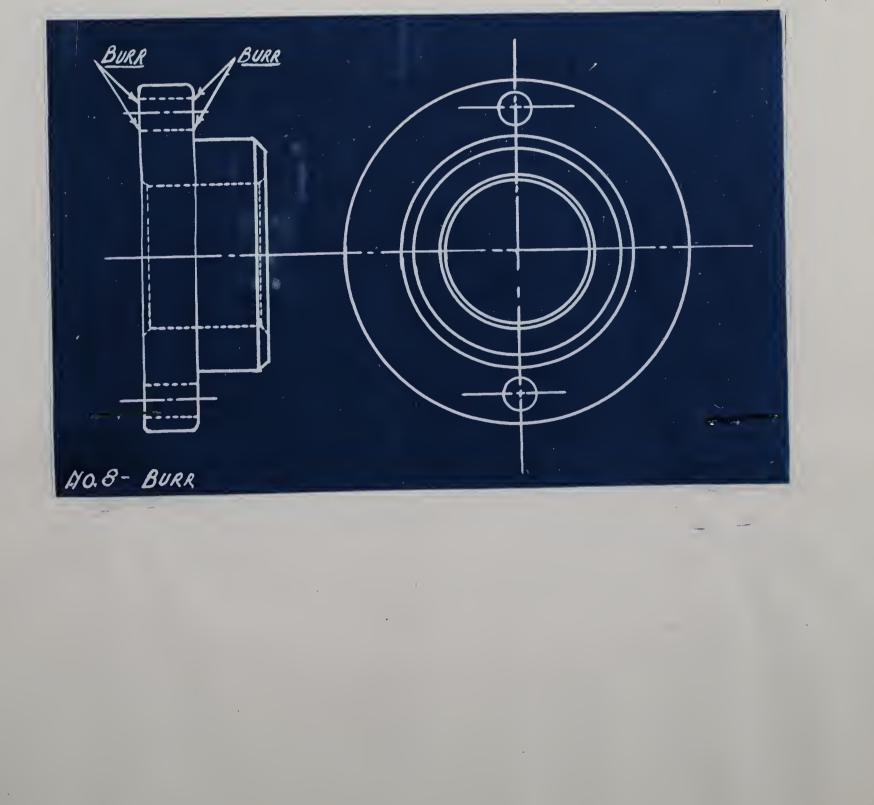
PART NO.2001 PART NAME Adapter DEPT NO. H.S.T.S. Drilling for MATERIAL tapped holes OPER.NO.9 SHEET NO.1 NO.SHEETS 24 TYPE OF MACHINE Drill press
