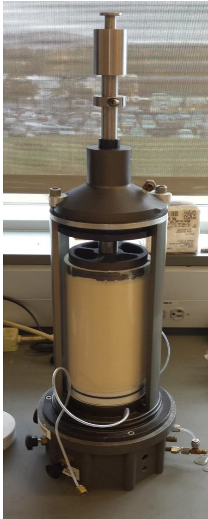
Figure 3. 3 Consolidometer used to make cakes of test soil 50S50K
