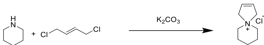
Scheme 7.3. Synthesis of 6-Azonia-spiro[5,4]decene chloride.
