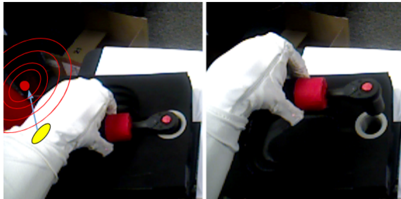
Figure 5.2. Example of a robot-proprioceptive action ( a_{RP} ) that extracts the ratchet.
