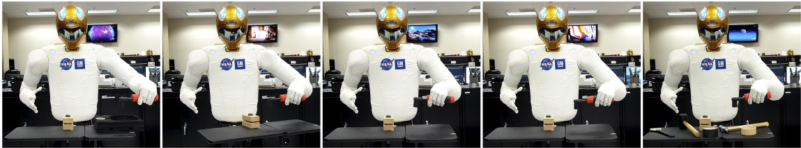
Figure 5.11. Corner case initial settings for mating the socket with the bolt. Note that in the 3rd and 4th image the in-hand ratchet positions are different.
