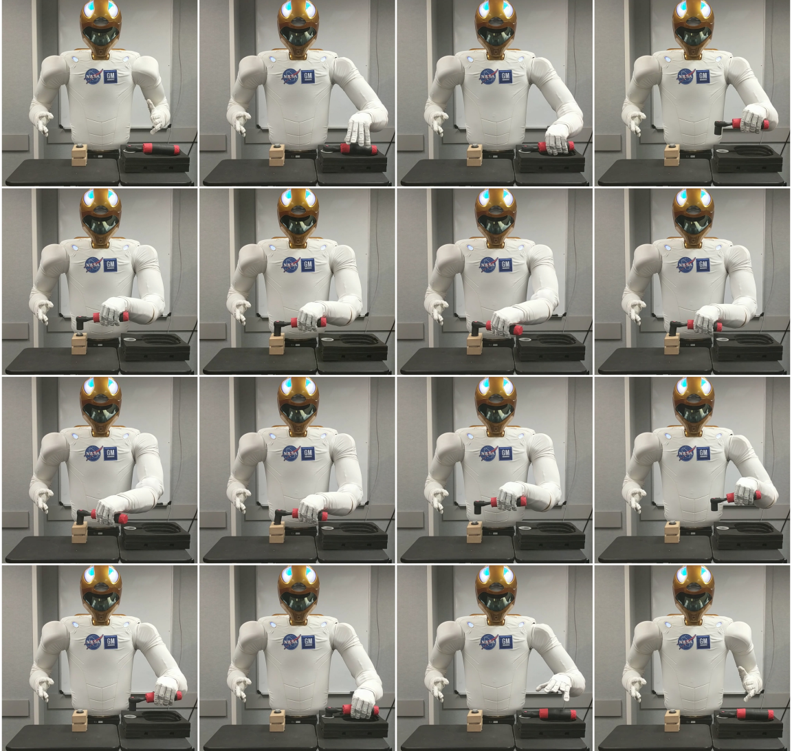
Figure 5.9. The ratchet task sequence performed by Robonaut-2. The images from left to right, then top to bottom, show a sequence of actions where Robonaut-2 grasps the ratchet, tightens a bolt on a platform, and puts the ratchet back into a tool holder.
