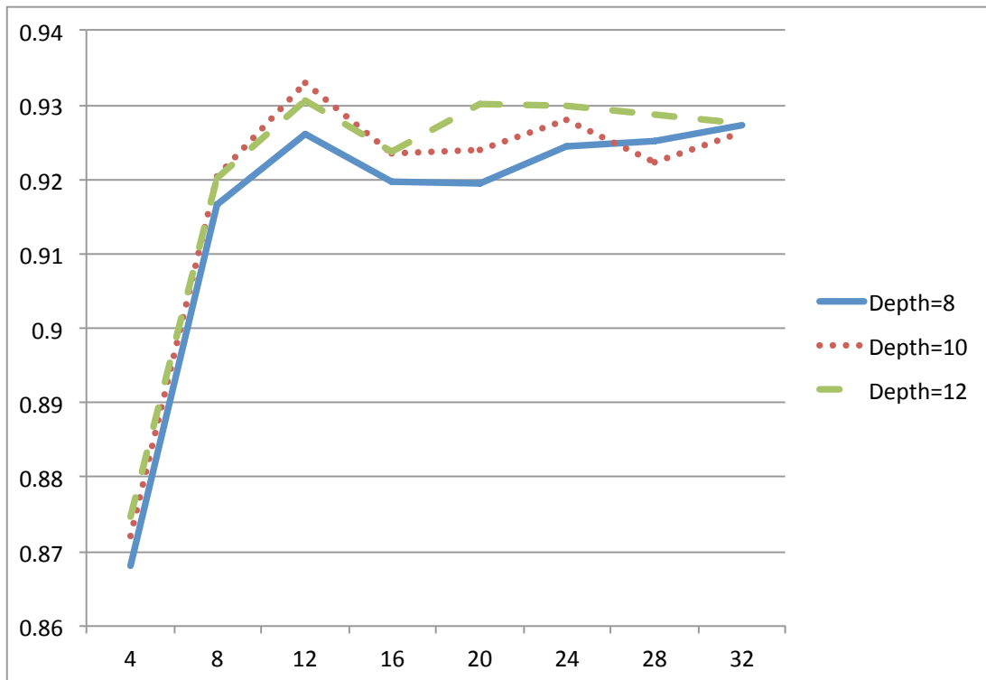
Figure 5.7: F-score for predicting the next phase for Python programs by offline cross-validated decision trees with 4, 8, 12, 16, 20, 24 and 32 selected features. The maximal depth of the decision trees is 8, 10, or 12.
