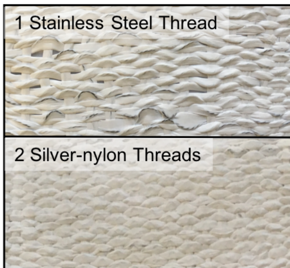
Figure 2.2: Thread(s) wrapped in low-density PTFE tape. Images show woven devices.
