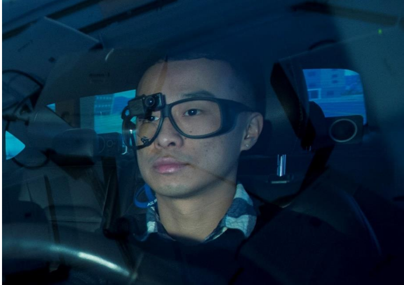
Figure 6: The eye tracker used to record glance behavior
