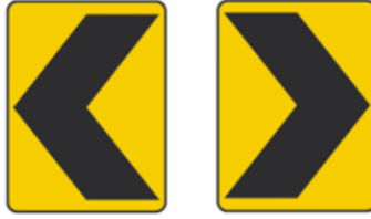
Figure 2 - Left and Right Curve Chevron sign
