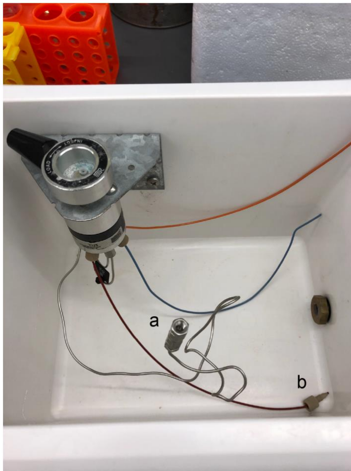
Figure 2.1. Icebox used to maintain minimum temperature during peptide separation step. Mass spectrometry sample was injected at the top of the valve. The metal connector (a) was connected to the output of the Waters HPLC and PEEK connector (b) was connected to the HPLC reverse phase column (not shown) for peptide separation. Both orange and blue lines are waste.
