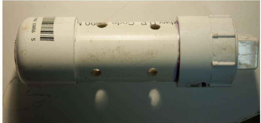
Figure A.2. A built logger housing showing the two rows of flow-through holes. The other four holes are located on the opposite side of the housing.
