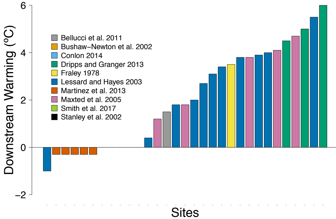
Figure 2.9 – Variation in warming magnitudes downstream of small dams reported across the literature, ordered from least to most warming. Positive bars indicate warmer downstream temperatures than upstream, negative bars indicate cooler downstream temperatures. Bars are color-coded by study (see in-figure legend for studies graphed), and each represents an individual dam site. Several sites (e.g., Bushaw-Newton et al. 2002, Stanley et al. 2002) simply reported no difference (i.e., no number values provided) and are plotted as a bar of 0 °C height.
