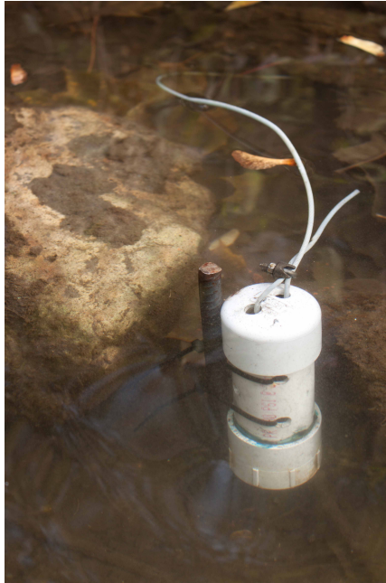
Figure A.4. A logger attached to a piece of rebar via two zip ties in a low gradient stream reach.
