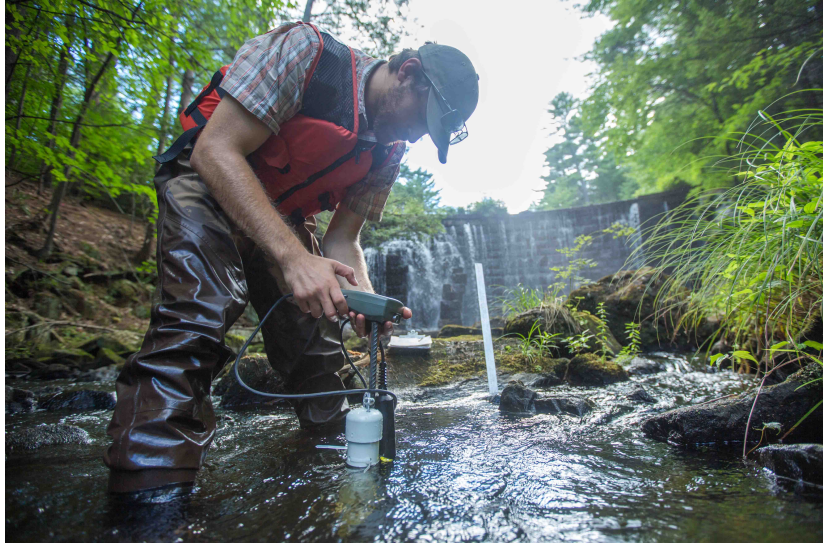
Figure B.7. Performing a reference calibration with the sonde placed immediately next to the installed dissolved oxygen logger.
