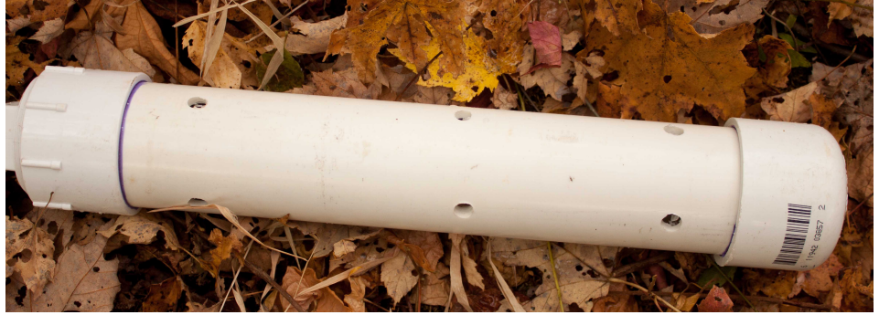
Figure B.2. An assembled logger housing showing the three rows of flow-through holes. The other six holes are on the opposite side of the housing.
