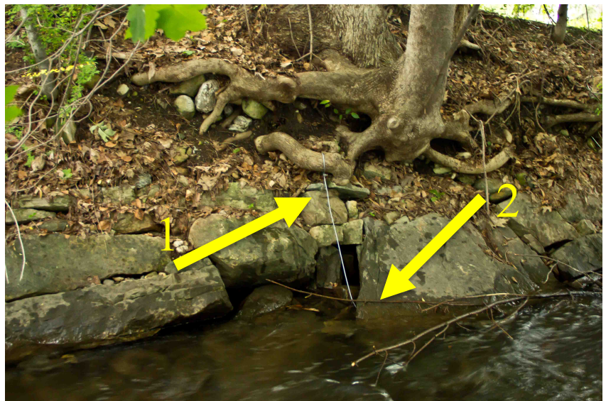
Figure A.3. Yellow arrow 1 indicates the permanent bank structure (root) being used to anchor the logger and housing in stream. Yellow arrow 2 indicates the large boulder and smaller rocks being used to protect and anchor the logger.
