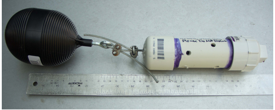
Figure A.5. A logger housing attached beneath a float.
