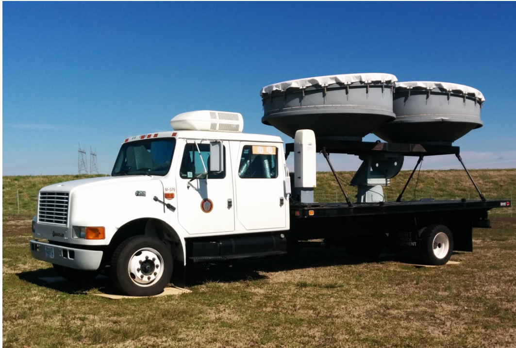
Figure 1.1. Picture of the UMass FMCW profiler at the 2016 deployment site during the Vortex Southeast experiment.
