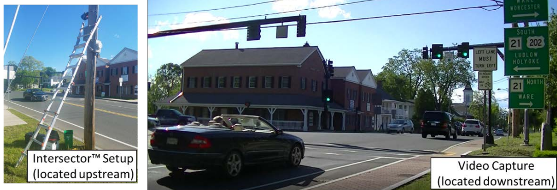
Figure 12 Intersector™ Setup with Video Capture taken in Western MA
