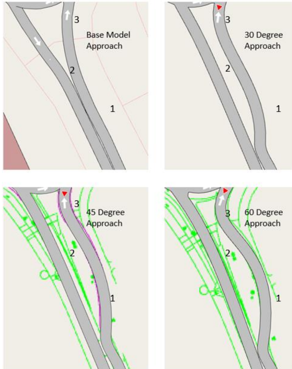
Figure 11: Distance Ranges marked on the Base and Experimental models on GRC approach
