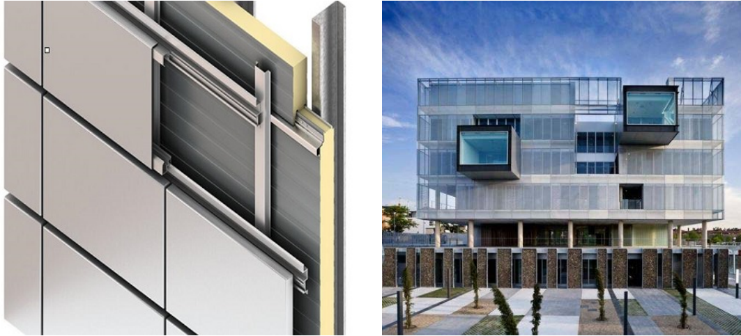
Figure 36 (Left) - Aluminum cladding system. 68 Figure 37 (Right) - Comisaria Fuencarral, by Voluar Arquitectos. 69
