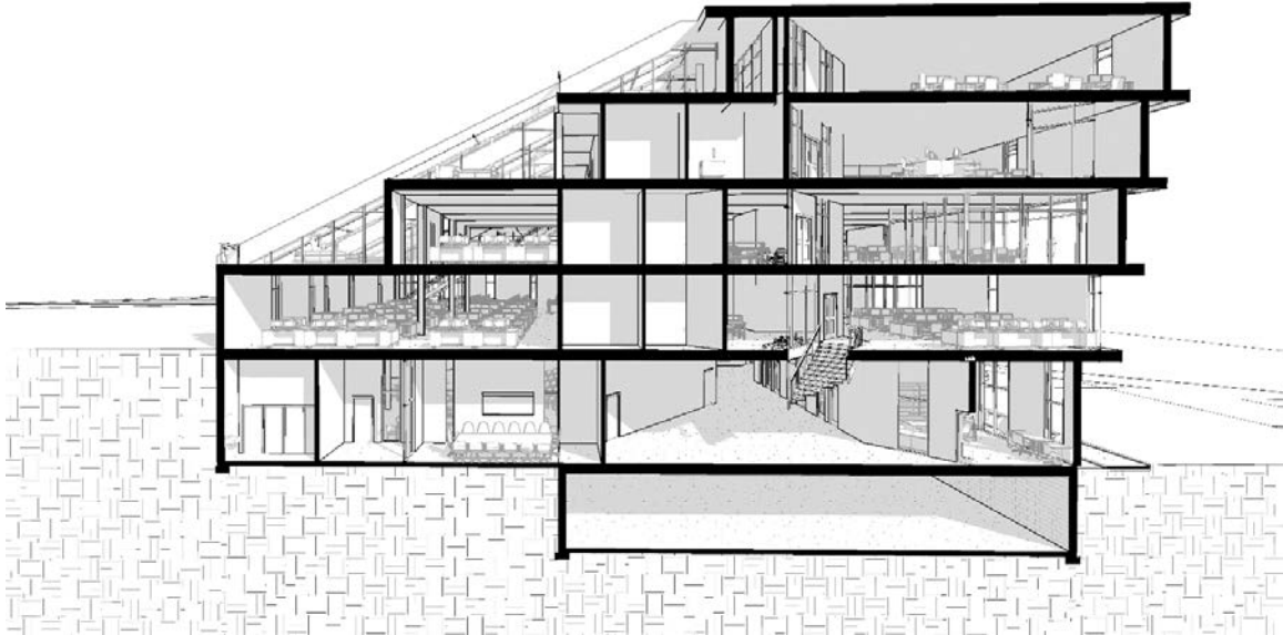
Figure 38 - Northwest Sectional Perspective, showing cantilevered northeast façade and angled southwest façade with exterior walkouts
