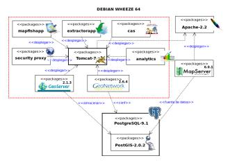
The IDE-EPB software architecture is based on geOrchestra for the management of GI, but also includes other components for all side infrastructure. In every part of the project, free software is exclusively used.
