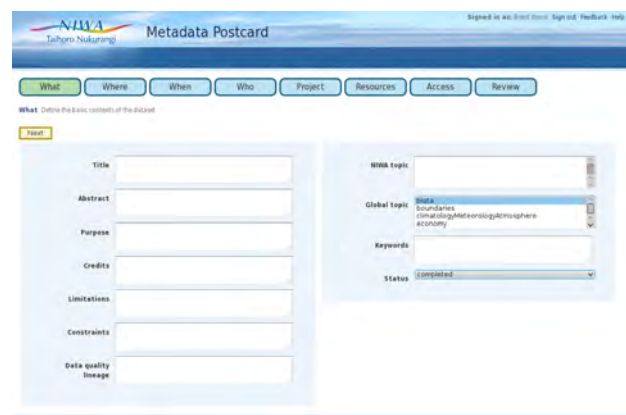
Figure 7: The NIWA postcard tool provides a user friendly interface for metadata entry. Tabs break up the content into subject areas, pick lists provide a simple controlled vocabularies for appropriate fields, The tool automatically emails NIWA's metadata curator of each record entered. The curator then checks the new record meets NIWA guidelines before enabling public access to it.
