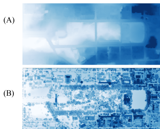
Figure 3. LiDAR data products used include (A) Digital Terrain Model (DTM) and (B) Digital Surface Model (DSM)
