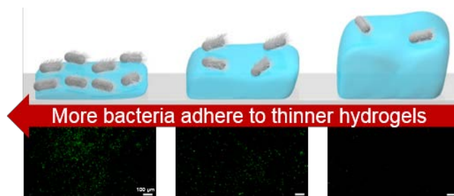
Figure 16: The mechanically sensitive adhesion of bacteria to PEG hydrogels is sensitive to the thickness of the hydrogel.
