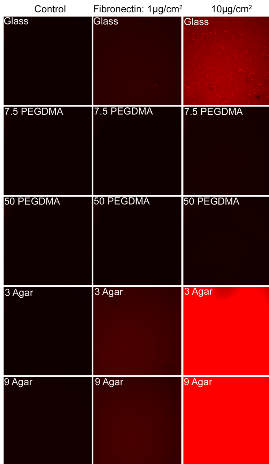
Figure 12: A qualitative protein adsorption assay was conducted using (left to right column) PBS only (control) and florescently labelled Fibronectin at two concentrations: 1 \mu\text{g}/\text{cm}^2 and 10 \mu\text{g}/\text{cm}^2 . No florescence was detected on PEG hydrogels, whereas protein readily adhered to glass and agar hydrogels. Representative confocal micrographs are presented.
