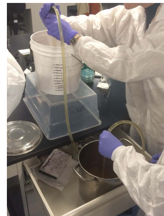
Figure 1: This is an example of a wort transfer setup using a cane and tubing to siphon beer with minimal introduction of oxygen and little transfer of insoluble waste products.
