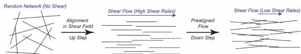
Figure 4.2: Alignment of CNTs during shear flow. The initially random CNT network aligns in the direction of flow as shearing forces are applied (Up step in thixotropic loop). At the highest shear rates the CNTs are aligned in the direction of flow and the viscosity of the fluid is low. On the Down step in the thixotropic loop, the CNTs are still roughly aligned in the direction of flow but they are able to interact as shear rate decreases, thus reinforcing the composite and raising viscosity.
