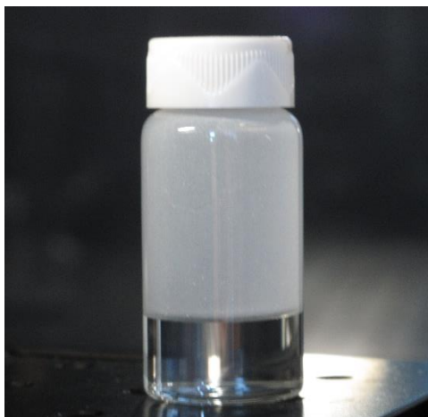
Figure B.1. 1 \mu\text{m} PTFE powder that has been vigorously shaken with 5 mL water in a Fisher scintillation vial. The opaque particle film coats the wetted walls of the glass. This film exhibits elastic behavior and will climb the walls if it is rinsed down.
