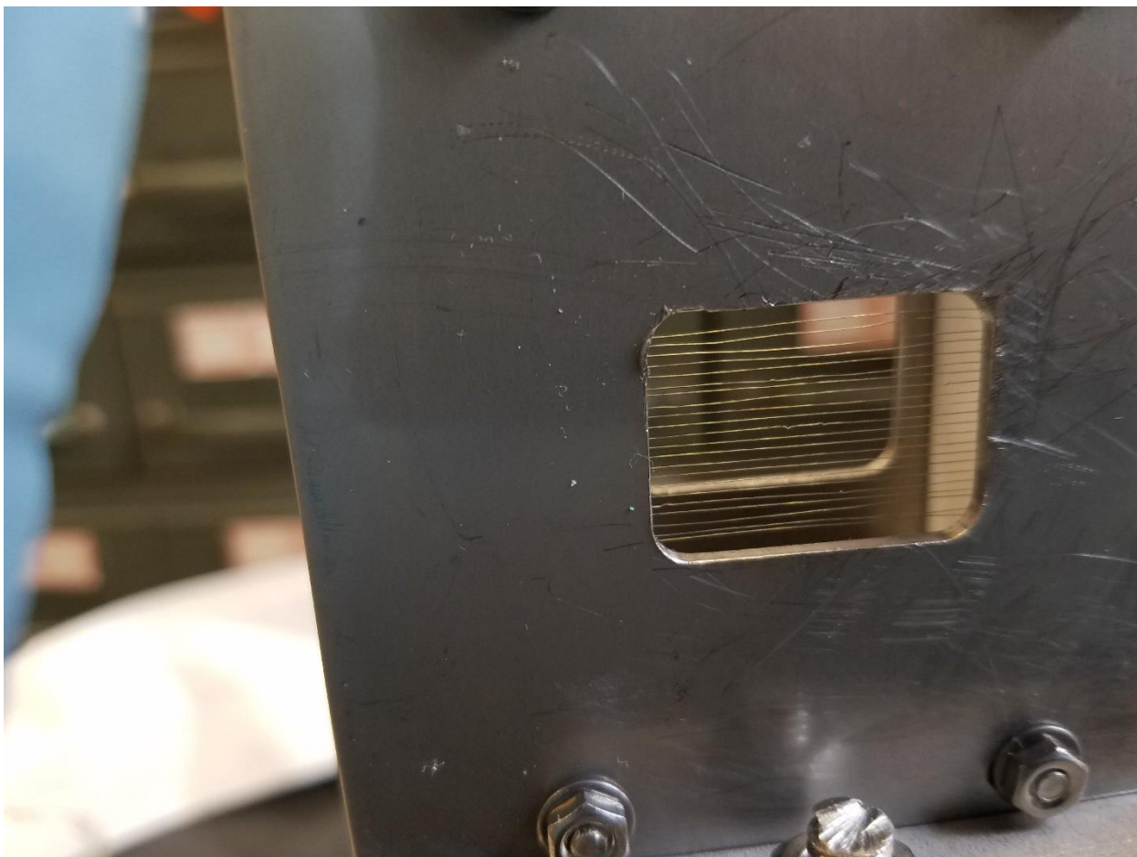
Figure 5.3: Custom mass gate after complete assembly. In this photo, the structure seen in Figure 5.2 is fully assembled and the is mounted between two stainless steel plates kept at ground potential. The final mounting and tightening of the plates results in the wires being fully tensioned. The molecular beam passes through the gap in the middle but purposely goes wide of the device when returning from the reflectron before arriving at the detector.
