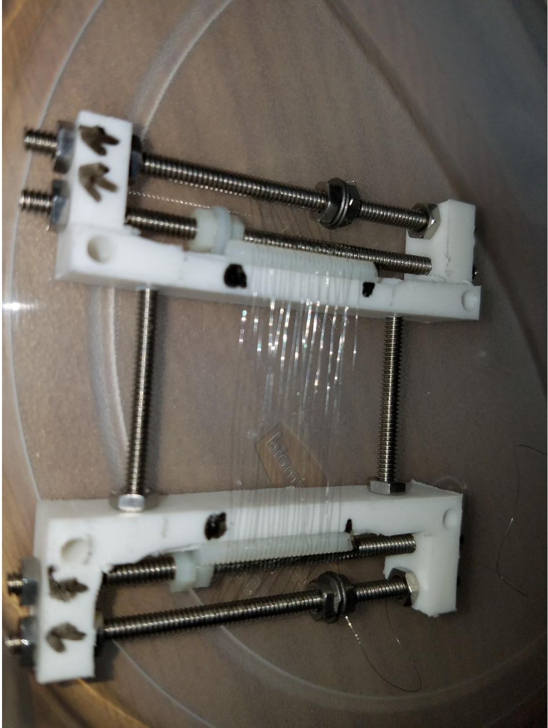
Figure 5.2: Custom mass gate structure before complete assembly. The wires are wrapped along metal and plastic screws to hold the lines in place as the mass gate will not function if they touch or are too close. The wires are ordered so that a positive pulse (coming from a wire that inserts between the nuts and the outer plastic for the metal rods) goes through the first wire on the left with the next wire having a negative pulse, and the wire after that again being positive and this pattern repeats across the lines. The main body is made from nylon, and the nuts can be adjusted to keep strong tension on the wires. In the photo, they are not yet fully tensioned.
