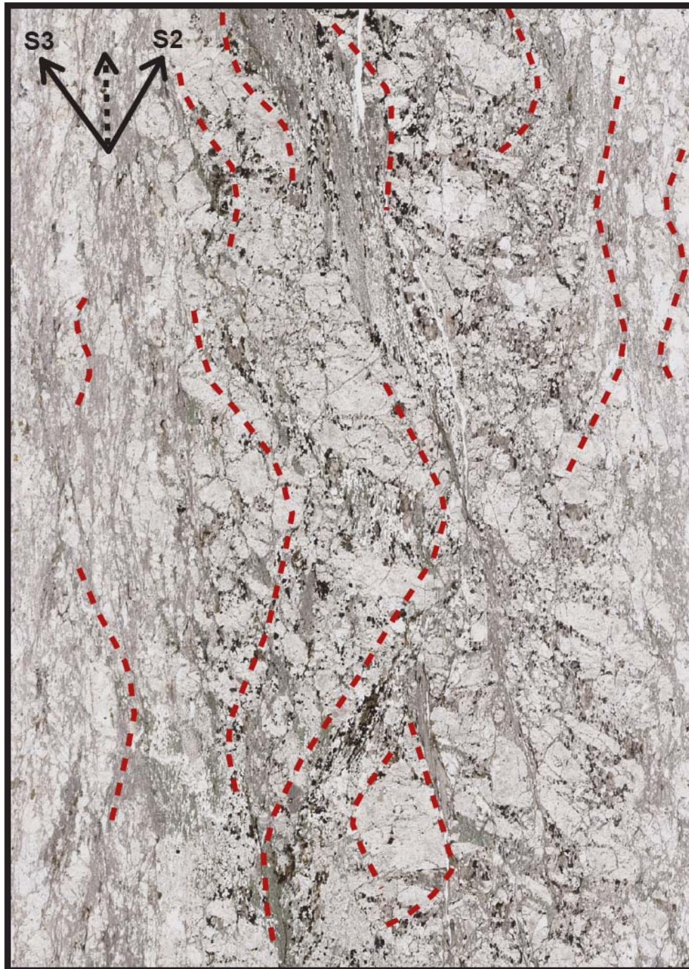
Figure 4.16. This thin section from the D3 high strain zone in the Maquinita Formation granodiorite shows the interaction of S2 and S3 to create the composite S2-S3 fabric (sample P06NM22; vertical section perpendicular to main foliation: 269, 84N).
