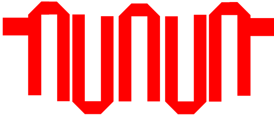
Figure 3-3 - Hairpin Distributed Element Filter Topology Example
