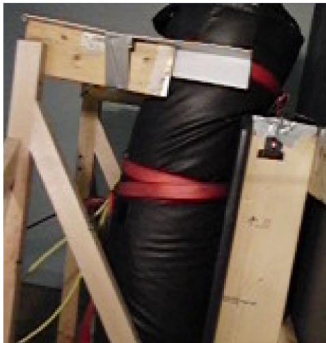
Figure 38: Unsupported upper segment of human model folding on top of wooden grill.
