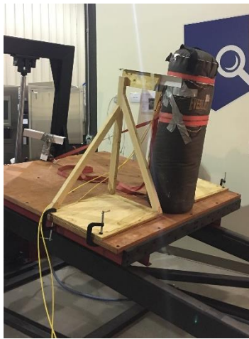
Figure 35: Pilot study human model configuration setup.
