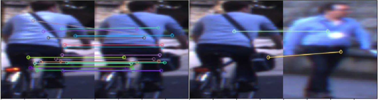
Figure 8: The Performance of the ORB on matching same object and different object
