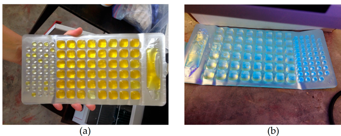
Figure 5. IDEXX Colilert-18 Quanti-Trays: (a) water sample testing positive for coliform; (b) water sample under UV light, testing positive for E. coli .
