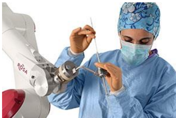
Figure 14: ROSA® stereo EEG Robot Allows for Accurate and Steady Placement of Depth Electrodes
