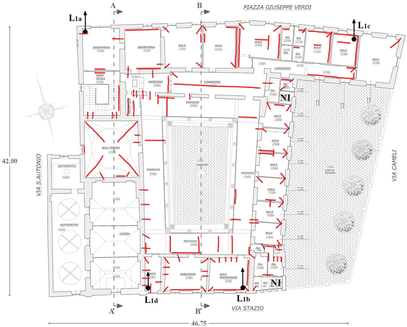
Figure 2. First floor plan. Crack pattern after the October 30 th event on the original survey by Ninni et al. (2014). All measures in m. NI = Not inspected, Li = acquisition point of ambient velocities
