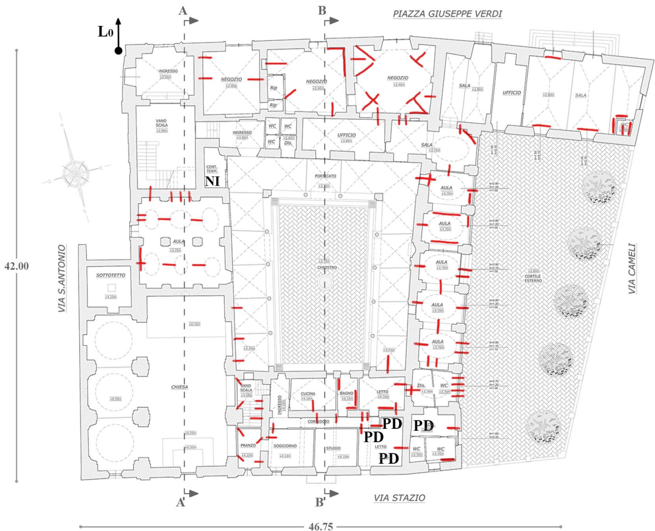
Figure 1. Ground floor (piazza Giuseppe Verdi) plan. Crack pattern after the October 30 th event on the original survey by Ninni et al. (2014). All measures in m. NI = Not inspected, PD = plaster delamination, Li = acquisition point of ambient velocities
