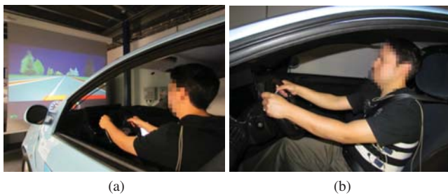
FIGURE 1. Measurement setup for driver drowsiness detection at IBV facilities. (a) Driving simulator room: front screen and car bodywork. (b) Participant wore three RIP bands around: abdomen, diaphragm and chest.
