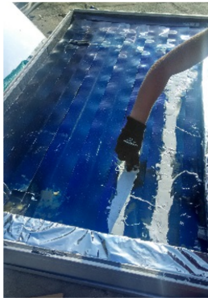
Figure 11: Application of the thermal paste on the copper fin of the thermal collector.
