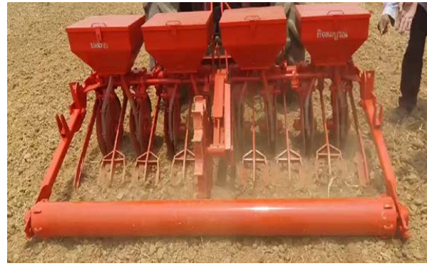
Figure 2: Thai rice farmer sowing seed by using a power tiller-operated seeder (Drill dry seeding)
