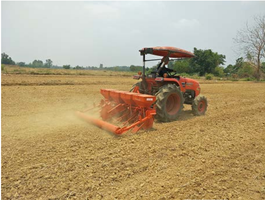
Testing power tiller-operated seeder (PTOS) at Phetchabun province
