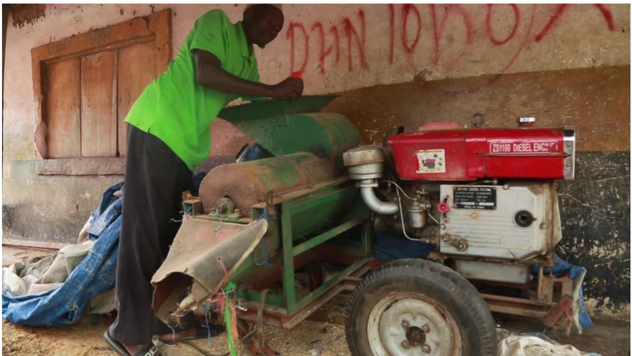
Kassim standing next to his 16-hpr maize shelling machine. Photo credit: Audifas Gasper/IITA.
