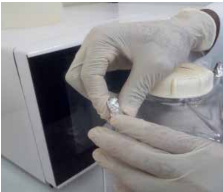
Plate 23. Top: Tight closing of medium vessel; Bottom: Covering of air and media connectors with foil
