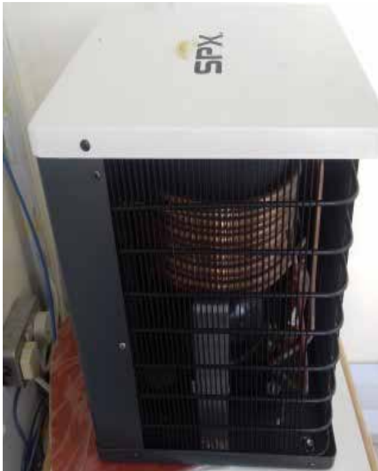
Plate 19. Air compressor (Top) and air dryer (Bottom) for the SETIS™ Type Temporary Immersion Bioreactor system.
