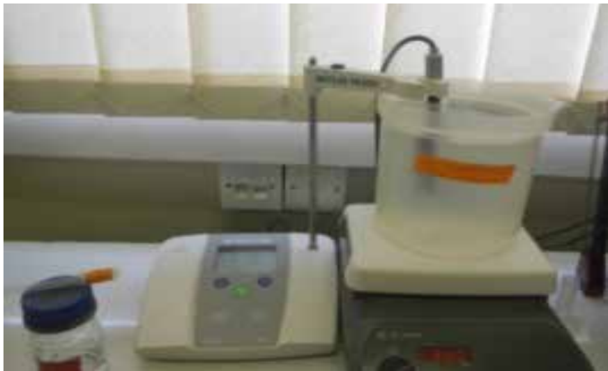
Plate 8. Preparation of medium for in vitro culture of explants. Top: Stirring of medium constituents and reading of pH; Bottom (Left): Dispensing of medium into culture vessels; Right: Autoclave for medium sterilization.
