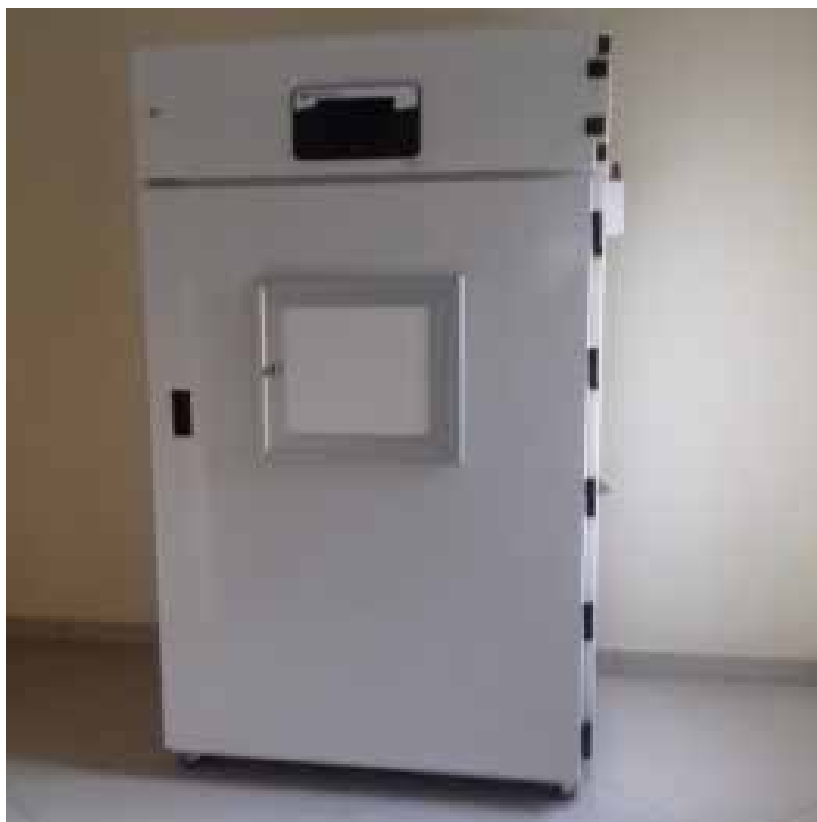
Plate 11. Temperature and humidity-controlled growth cabinet for heat treatment to clean plantlets from viruses.
