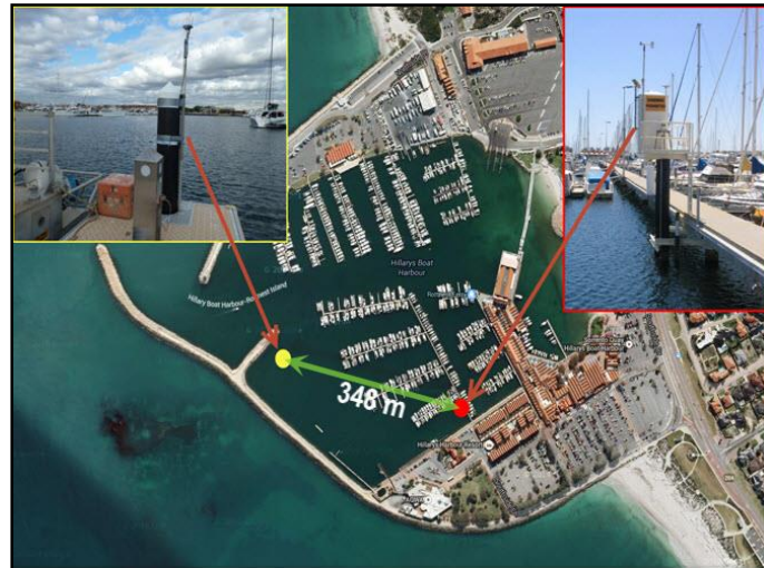
Figure 1. Hillarys Tide Gauge (red circle) and GNSS water level height station (yellow circle) [Fugro, 2014].
