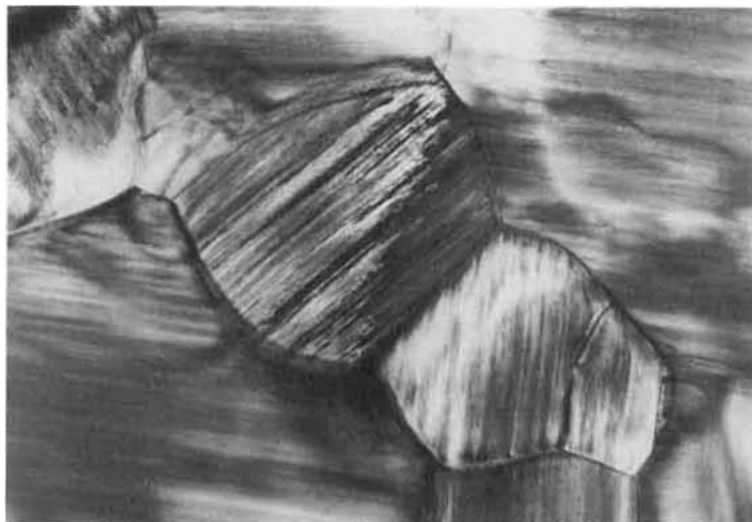
Fig 2.4 TEM micrograph showing twinned domain pattern in a single grain of NTO, sintered at 1450^\circ\text{C} (doped with 3 mole % \text{Nb}_2\text{O}_5 ) [2].
