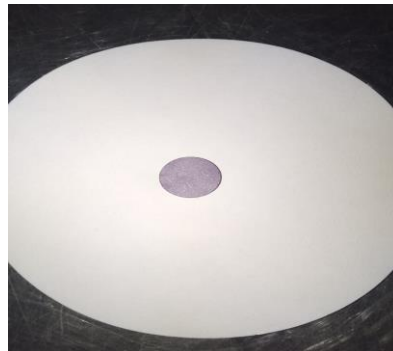
Image3.8. of pellet sintered at 1400°C for 5 hours using high temperature furnace with heating and cooling rates are 5°C/min.
