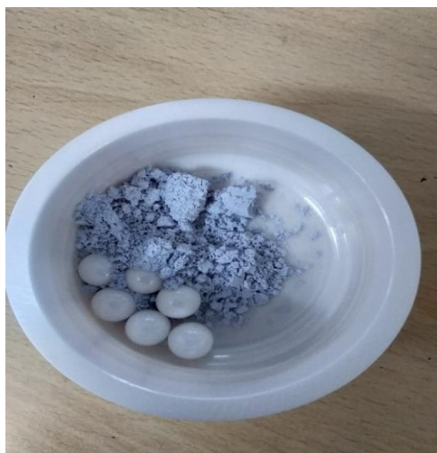
Fig 3.6. shows NTO sample within ball milling cylindrical vessel. Wet Ball milling (mixed 2-propanol) of sample was done with 200 rpm for 11 hours to make fine powder.
