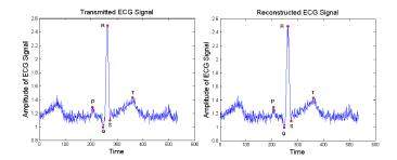
Fig. 8: Transmitted and Received ECG Signal through AWGN
