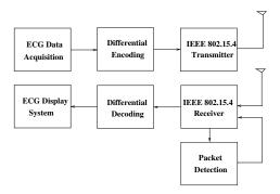
Fig. 3: Overall System Architecture
