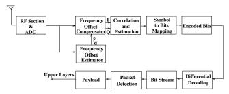
Fig. 6: Proposed IEEE 802.15.4 Receiver for ECG Data Transmission
