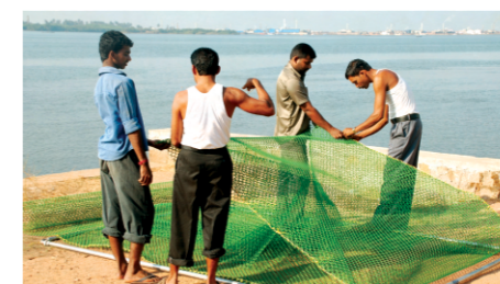
Fig. 4. Outer net fabrication using Netlon material
