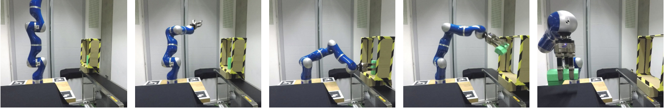
Fig. 8: Experiment on robot hardware H_2 : fetching an object placed inside of a shelf on a moving conveyor belt.
