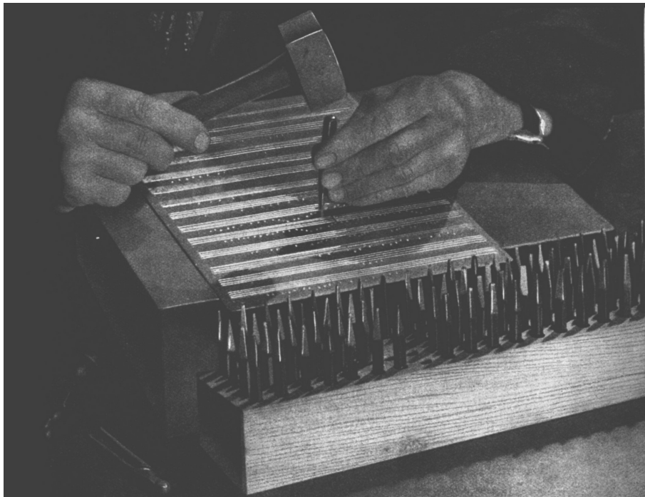
Figure 2.4: The traditional hand-engraving process [39]
