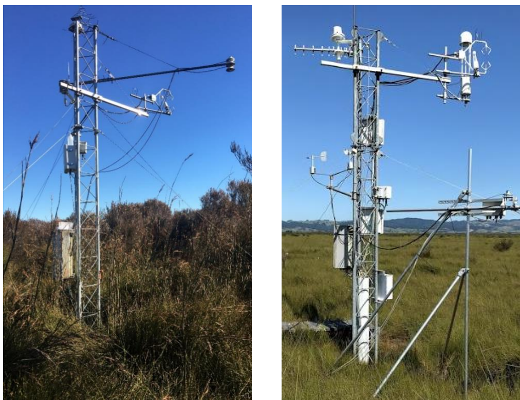
Figure 3.9: EC tower sites. Moanatuatua (left) and Kopuatai (right).
