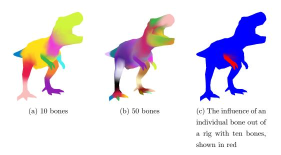
Figure 5.3: The influence of different bones visualized with separate colors
