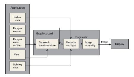
Figure 2.2: The computer graphics pipeline (Hughes et al., 2014)
