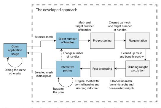
Figure 3.1: The developed mesh processing pipeline (the phases with user interaction are drawn in blue and automated phases in light gray)
