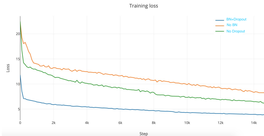
Figure 7.1: Training loss with and without batch normalization and dropout.
