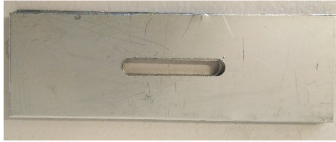
Figure 30 Slots in the stainless steel plate
