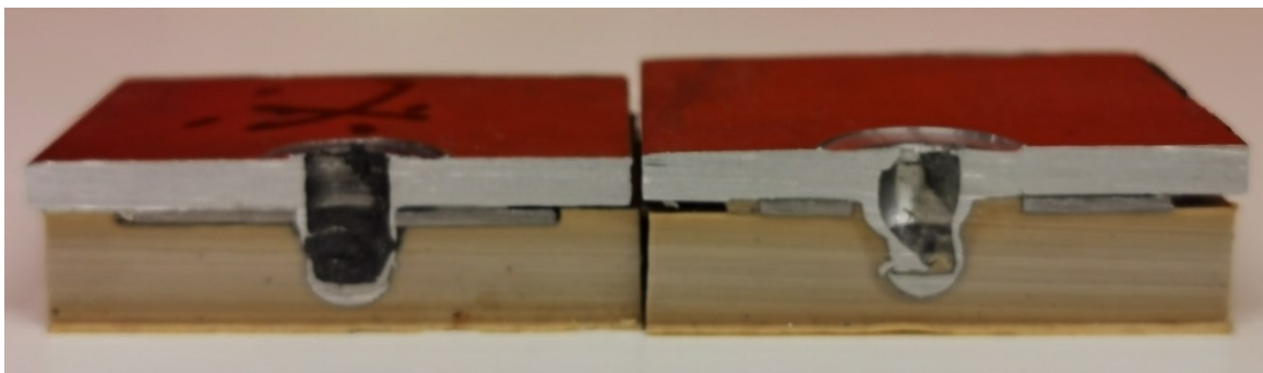
Figure 40 Welding without stationary shoulder
