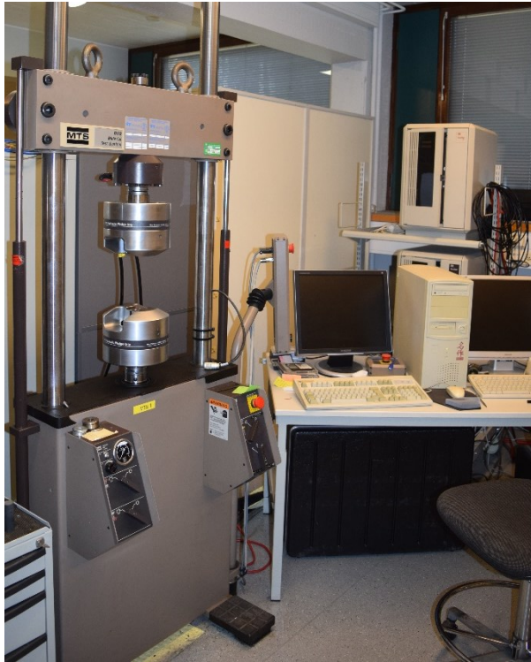
Figure 26 MTS Landmark 810 Material Testing Machine
