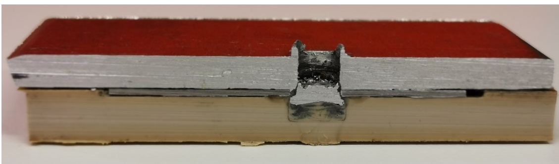
Figure 42 Weld obtained using a stationary shoulder
