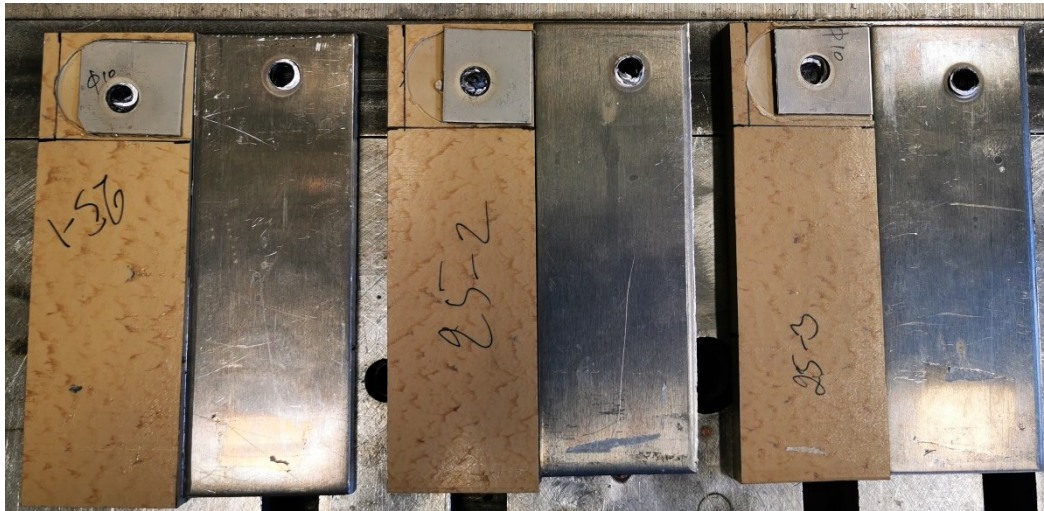
Figure 45 Workpieces after tensile shear testing
