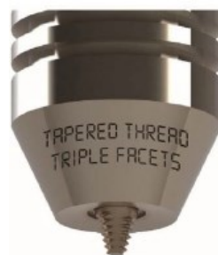
Figure 18 Friction Stir lap welding tool used for joining aluminium and PEEK [59]
