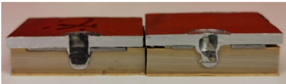
Figure 39 Welding done using the new clamping system
