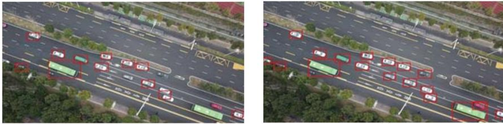
Figure 2.7: YOLO v2 detection result (left) and optimal dense YOLO method detection result (right) (Zhi Xu et al. 2018)
