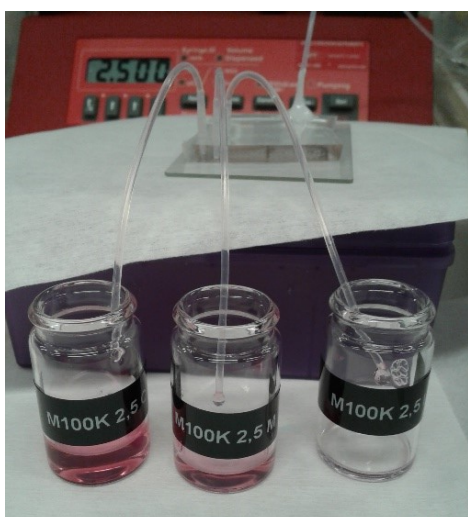
Figure 31 Syringe pump in the background is pumping 2,5 ml/min to assembled Labyrinth chip during cell medium test. Sample is gathered to vials; outer, middle and inner outlets.
