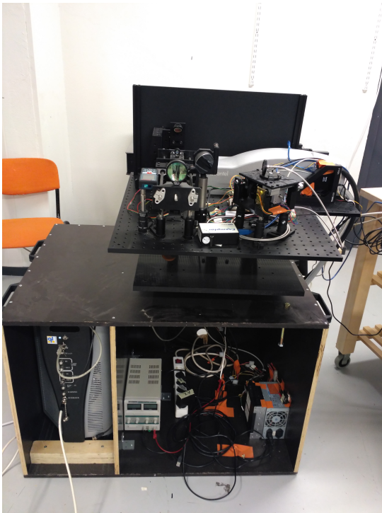
Figure B1: Mobile tunnel wall LIBS scanner device without casing
