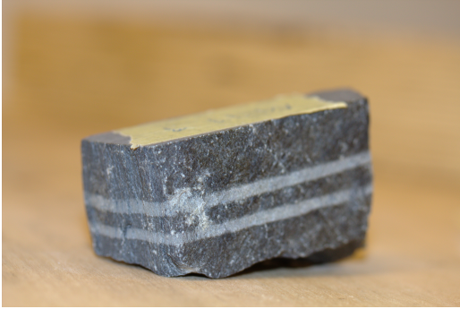
Figure 8.1: Kittilä Au mine rock sample with burn marks from 2 measurement series.
