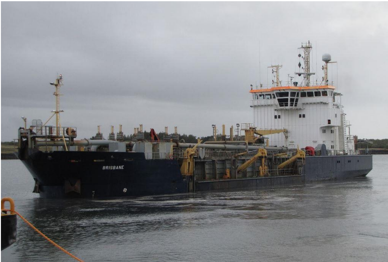
Figure 2: Trailing suction hopper dredger (TSHD) Brisbane (Dredging Today, 2015)
