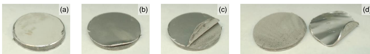
Figure 1 – Sample preparation process (a) sample as received from building (b) incision along the intersection of core and metal skin (c) beginning of peeling using pliers (d) metal skin completely removed.
