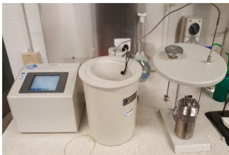
Figure 4 – Bomb calorimeter using a Parr Instruments (Moline, USA) Calorimetric Thermometer Model 6772.
