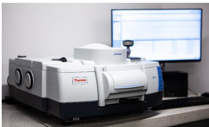
Figure 2 – Thermo Fisher Scientific Nicolet iS50 FTIR spectrometer with Raman and diamond ATR accessory.
