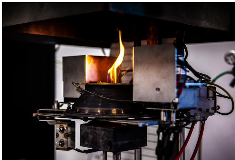
Figure 5 – Cone calorimeter (Fire Testing Technology, UK) during operation.
