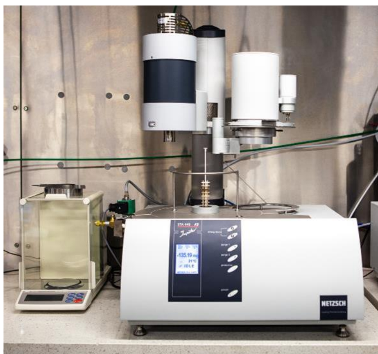
Figure 3 – Netzsch Jupiter STA449 F3 used for analysing the thermal degradation of all samples.
